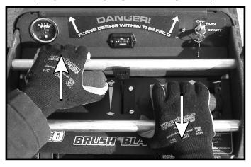
Grab the left steering control handle with your left hand and push forward while at the same time grabbing the right steering control handle with your right hand and pulling back. This will spin the machine right, without mowing forward.
